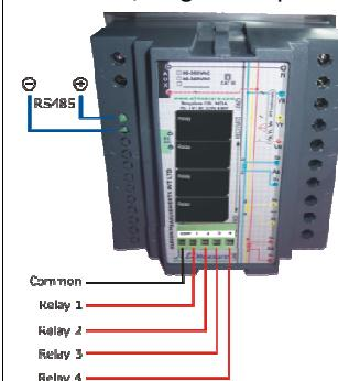
Note: Connections to the terminals located at the rear side of the unit is to be made by using preferably 12 to 14 SWG (2.6mm<sup>2</sup> to 2.0mm<sup>2</sup>) industrial grade wire. Relay rating No contact SPST. 250VAC / 30VDC @ 2 Amps resistive.
