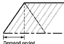
**Block Window:** This window slides every demand period. It has to be synchronized to EB meter manually. It will return to zero at the end of demand period. This can be used for the fairly stable load. The graphical representation of block window.
