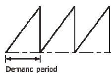
**Forecast Demand Control:** Forecast demand control is more suitable for sliding window technique. This control predicts the rising demand before the set time (Forecast Interval) and gives the alarm/annunciation for pro active action. The user can then shed some non-critical loads. (Additional load information is available in Demand page). 4 relays are used to control the demand
